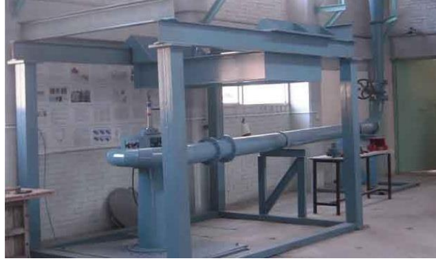
Figure 2. Francis Turbine Test Rig in Turbine Testing Lab (TTL), KU
